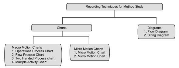
Fig. 7.4 Recording techniques for method study
