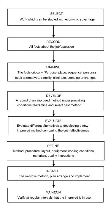
Fig. 7.3. Method study procedure
